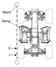
The rear measurement should be 1/16"-1/8" (2-3 mm) more than the front measurement on each side of the vehicle to obtain the recommended 1/8" to 1/4" (3-6 mm) toe out alignment.
